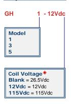
\*Order the relay with the coil voltage in the part number as shown above. The coil voltage will appear on the coil plate near the coil terminals rather than in the P/N on the relay.
